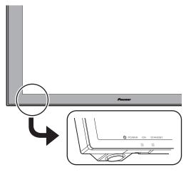
The lower left section of the display unit shown in the illustration above is the location of the MAIN POWER switch and certain parts required for display, and the contour involves a raised projection.
